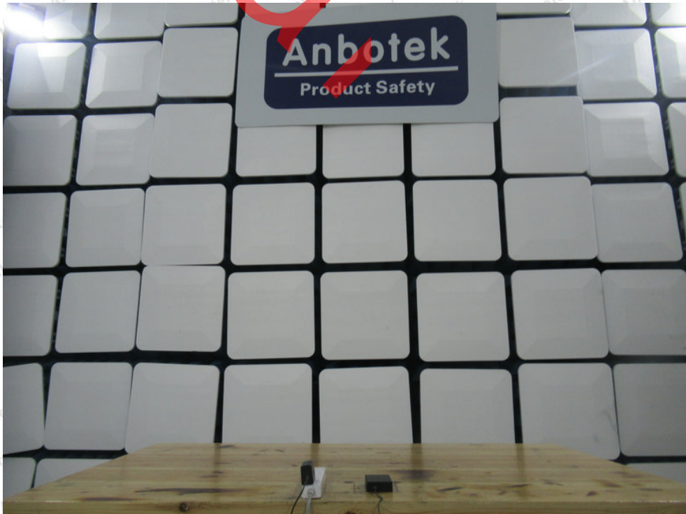
Photo of RF Field Strength Susceptibility Test
