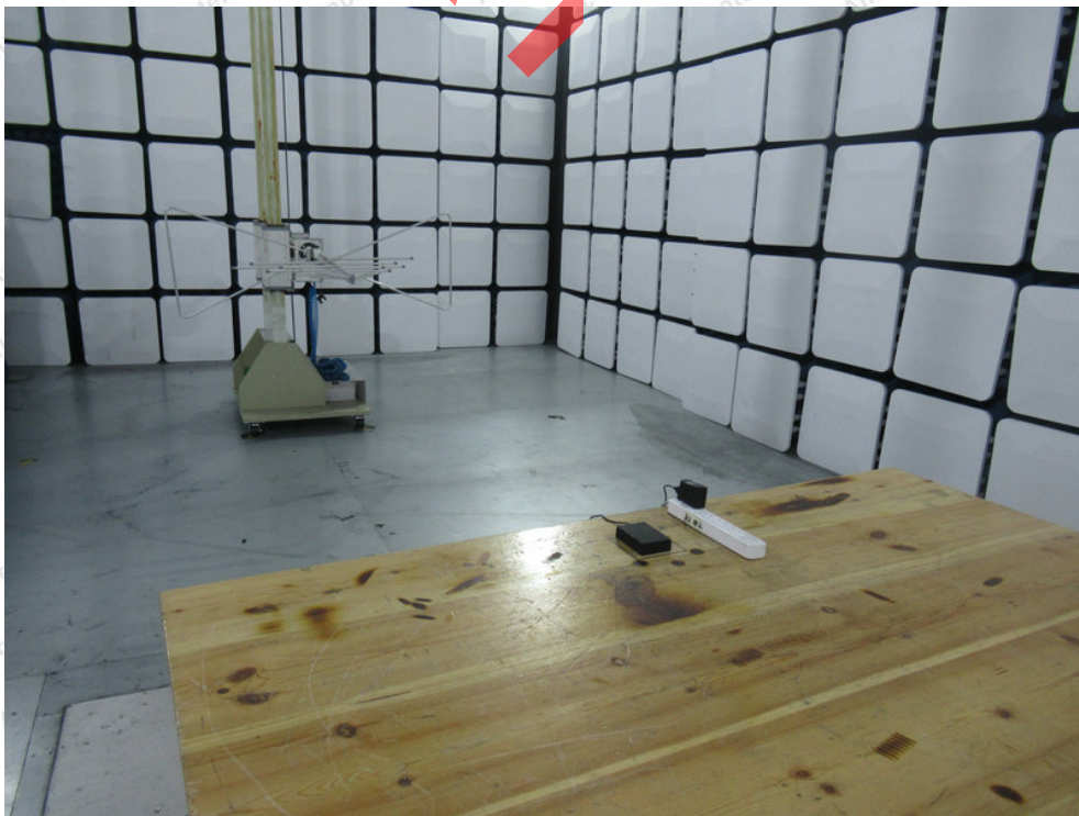
Photo of Radiation Emission Test
